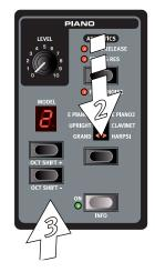
Changing any parameter on the Nord Piano 2 panel will immediately cause an asterisk to appear next to the current program number in the display.
