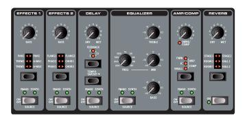
The Effects section of Nord Piano 2 can be used to process the pianos and the samples. It is programmable and you can configure your effects separately for each and every program. Some of the effects are mono in/Mono out and some are stereo in/stereo out. For each individual effect the channel configuration is stated in the related text.
