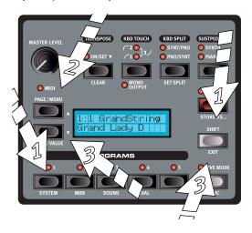
3 Set the memory protection to Off by pressing and holding Shift and then press the Down button.
