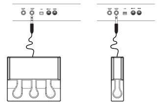
Connect the connector from the Nord Pedal to the Sustain Pedal connector on the Nord Piano 2.
